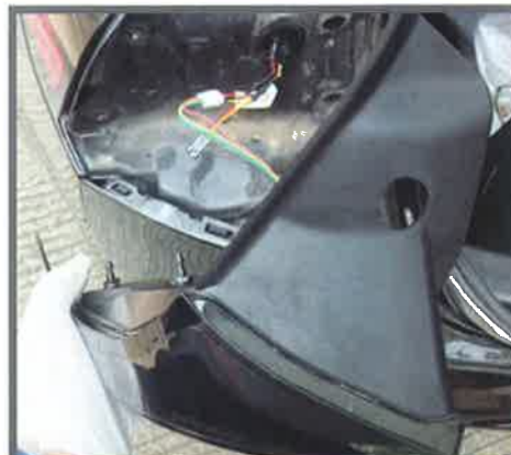
7. Replace the new bend lamp and restore the installation screws and connectors
