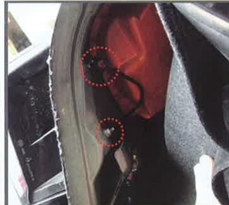
5. Break off the partition, remove 2 screws and unplug the connector
