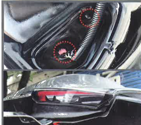
2. Remove the flat lamp: Unplug the connector, unscrew the screw (above), and remove the flat lamp with the rocker (below)
