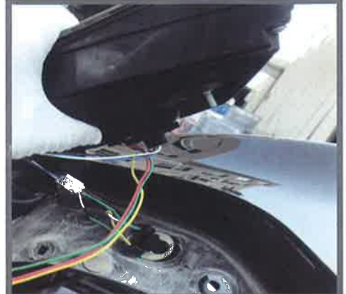
3. Replace with a new flat lamp and restore the installation screw connector
