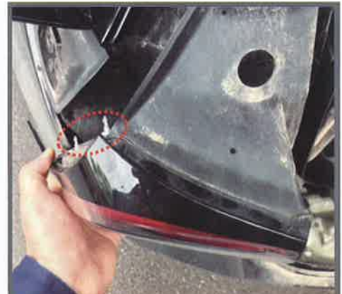
6. Use the prying plate to remove the set screw and then take out the bending lamp
