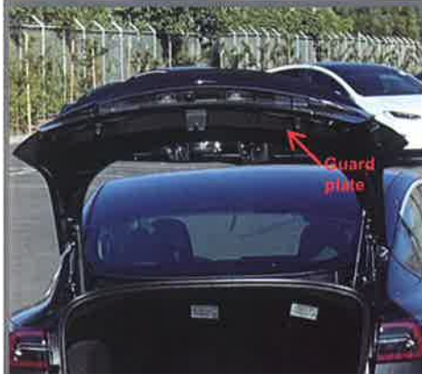
1. Open the trunk and break off the guard
